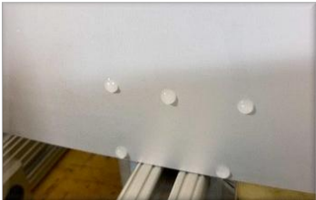
Sample of Ice De-bonding Test on Aluminum Substrate (NCI +MA +EC: 40 seconds)
